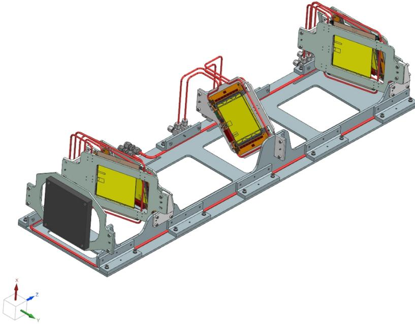
Figure 2.5: CAD Of a MUonE tracking detector ("station"). From left to right, along the  $z$  axis, the incoming CERN M2 beam hits the low-Z target electrons (in black). The paths of the scattered particles are then recorded by the 2S modules (in yellow) on the three detector plane pairs located behind the target.
