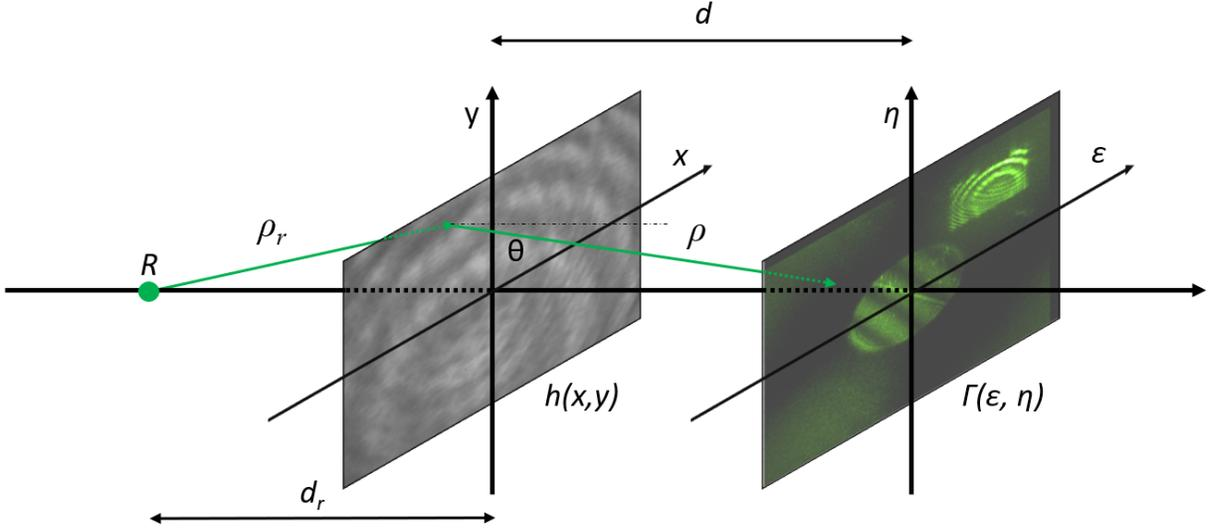
Figure 2.4: Holographic reconstruction scheme showing the re-illumination of the raw holographic data  $h(x, y)$  by the "reference" wave  $R$  at distance  $d_r$ . The reconstructed field  $\Gamma(\epsilon, \eta)$  is then formed at distance  $d$  from  $h(x, y)$ .
