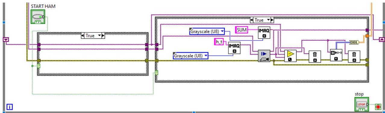
(b) Algorithm for image acquisition for the  $h_{t_n}$  with the last  $h_0$  continuously recalled within the while loop by the shift-register method. The two raw holographic images are subtracted and ready for reconstruction. (Condition value is "True")
