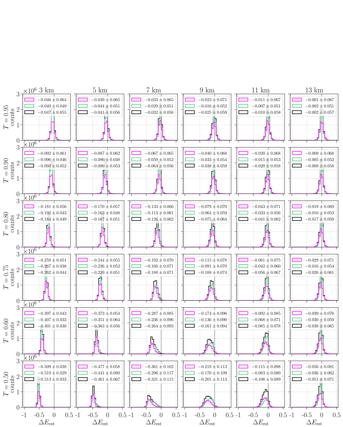
Figure 4.26: A distribution of \Delta E_{\text{est}} for CTAO-N and the corresponding subarrays. The colors black, green, and pink represent CTAO-N, 15 MSTs, and 4 LSTs, respectively. The column represents the height of the cloud, while the row represents the transmission of the cloud. For each case and array, the mean and width of the distribution are reported.
