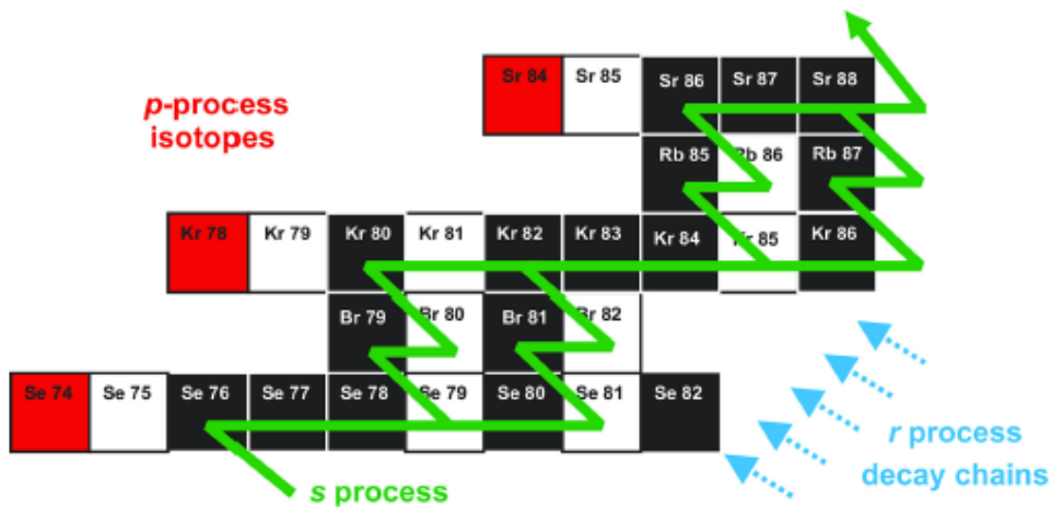
Figure 7: Diagram explaining s, r and p-process. Taken from [1, p. 330].
