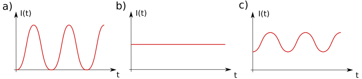
Figure 2. 16. Detector signal of a) linearly, b) circularly, and c) elliptically polarized beam at the detector.
