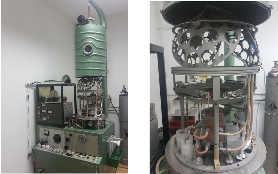
Figure 3. 3. Photo of the evaporation plant.
