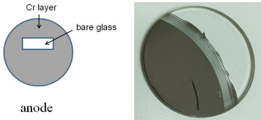
Figure 3. 1. Scheme of macro-structured (left) and photo of micro-structured anode (right).
