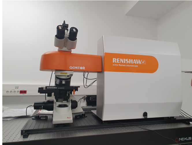
Figure 2.10: Photograph of commercial Renishaw in-via Raman confocal microscope.
